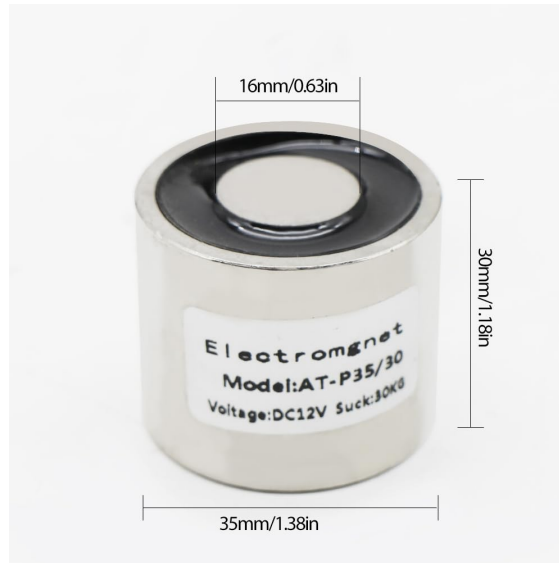
Figure 23: 35 * 30mm cylindrical electromagnet, capable of producing 300N (66lbs/30kg) of magnetic force. Four of these were used in the DLZ, meaning a 120kg UAV could be suspended upside down.
