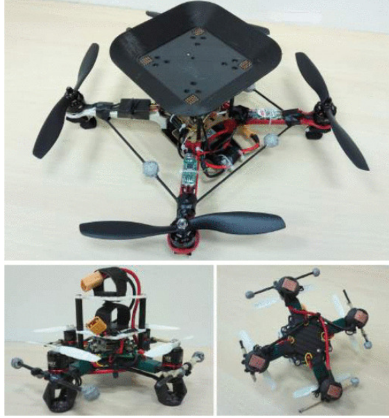
Figure 5: UAV prototype developed by Jain and Mueller showcasing the designs for a UAV with a docking system (top) to secure and draw current from a UAV with an external battery for charging (bottom).
