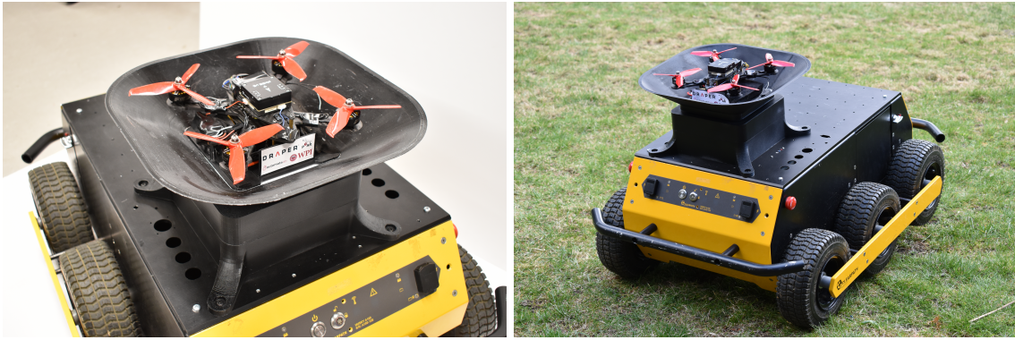
Figure 6: Full UAV-UGV docking and charging system, with our system's UAV docked and in charging mode. ClearPath Robotics Husky A100 UGV also pictured.
