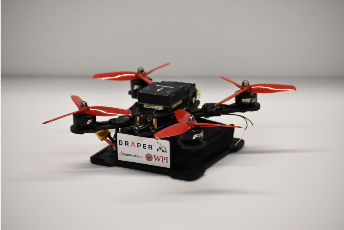
Figure 14: Our system’s UAV: an 8-inch, lithium-ion powered quadcopter with a custom 3D-printed landing foot to interface with the UGV’s dorsal landing zone (DLZ)
